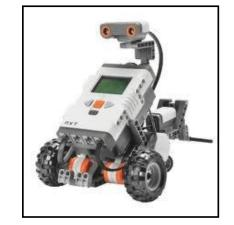
with the NXT robotic bricks. Motors and various sensors such as the ultrasonic, sound and touch sensors are connected to the bricks and programmed. Working with a partner, students will be challenged to follow plans to build machines as well as design their own projects. As they write, test and debug procedures for their projects, students will be using their creative and critical thinking skills.
